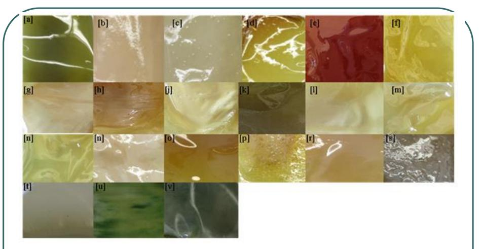
Pre-dissolving GA in dry DMAC affects the actions of GA, and the resulted membrane formation gives difference in terms of color and contact angle. For example, the membranes "n" and "s" were from PAA-DA. Even though, the membrane "n" is plastic-like transparent while the membrane "s" is opaque and dark-blue color with possessing higher contact angle;
