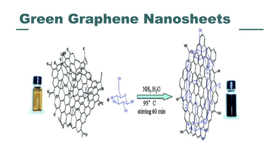
Chengzhou Zhu et al have developed a green approach to the synthesis of chemically converted graphene nanosheets (GNS) based on reducing sugars, such as glucose, fructose and sucrose using exfoliated graphite oxide (GO) as precursor.
