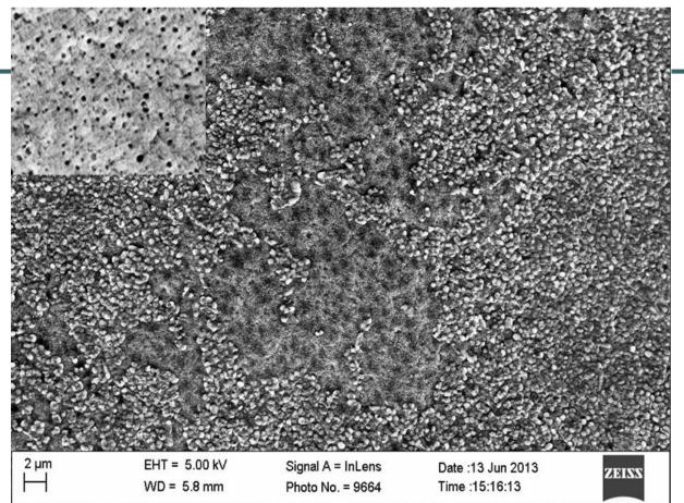
GA treated PAA-CS and PAA did not lose their surface integrity and pore-size distribution for disinfection of 1000 mL tap water containing 3 e8 Staphylococcus epidermidis, Escherichia coli and Citrobacter frenduii
