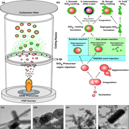
$\Box$ Potentially toxic nanomaterials are coated with a biologically inert layer of amorphous SiO<sub>2</sub>.
